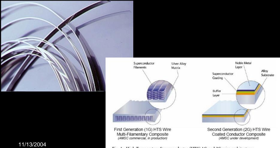
Fig. 1: High Temperature Superconductor (HTS) 1G and 2G wire architectures
