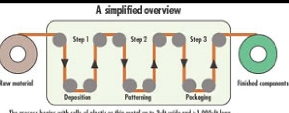
The process begins with rolls of plastic or thin metal up to 3-ft wide and >1,000-ft long. The media passes through processing chambers as silicon is layered on the surface. Finished goods might include memory, display, RFIDs, batteries, CPUs, and more.
